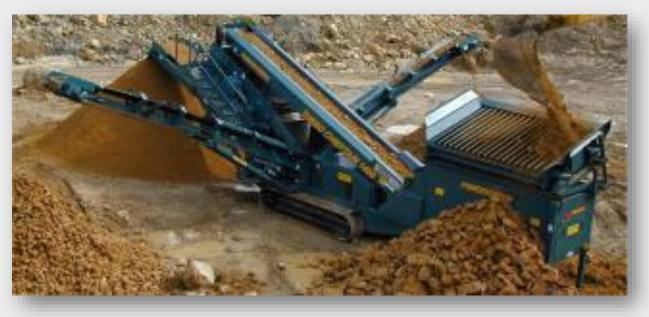
Higher Cost @ \$15,000-\$20,000/ month On tracks and folds for transport Good for high production High maintenance
