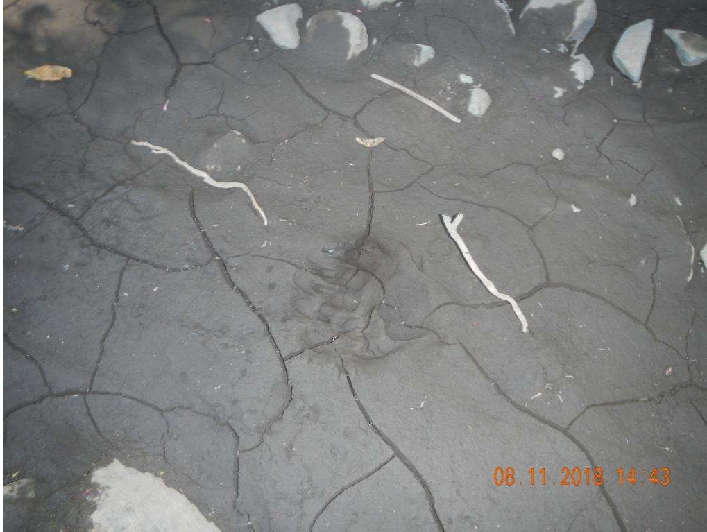
Picture 13 – Deposit of fine sediment (silt) from July 15 th , 2018 thunderstorm runoff event
