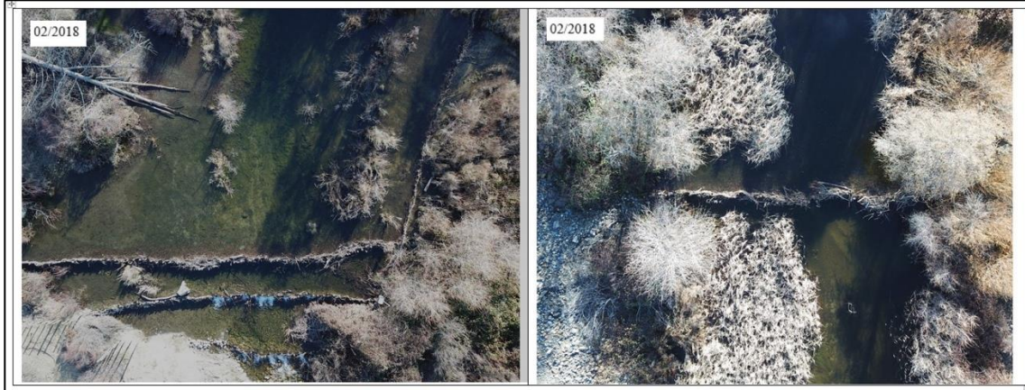
Figure 28. Landscape Photos from Sugar Creek restoration site. Left photo: Sugar BDA 1.0 with step BDAs 1.1 and 1.2, Side Channel 1 to the right and flowing from BDA 1.0 wing, and recent cottonwood fallen by beavers. Right photo: Sugar BDA 2.0
