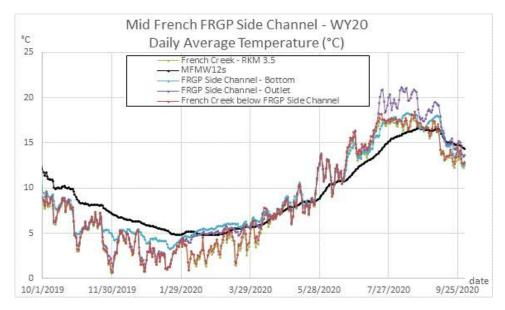
FIGURE 10. DAILY AVERAGE WATER TEMPERATURE (°C) - SIDE CHANNEL AND MID FRENCH CREEK - WY20.
