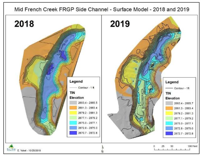
MAP 4. 2018 AS BUILT AND 2019 SURFACE MODELS OF SIDE CHANNEL.
