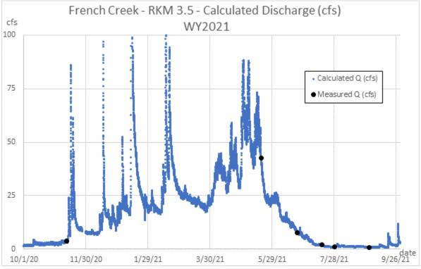
Figure 3 – Calculated and measured stream discharge (cfs) – French RKM 3.5 – WY2021
