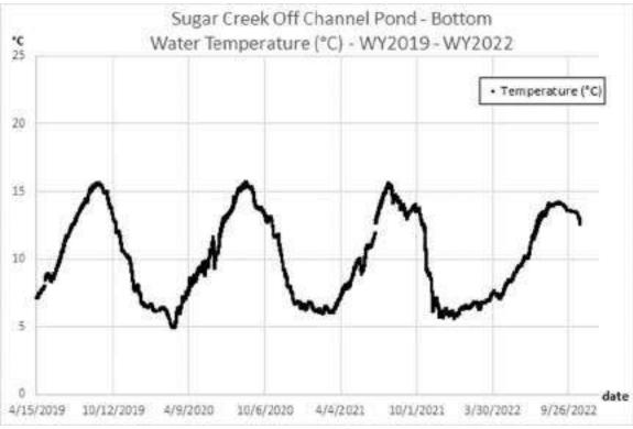
Figure 10. Continuous water temperature (°C) - Sugar Creek Off Channel Pond - Bottom.
