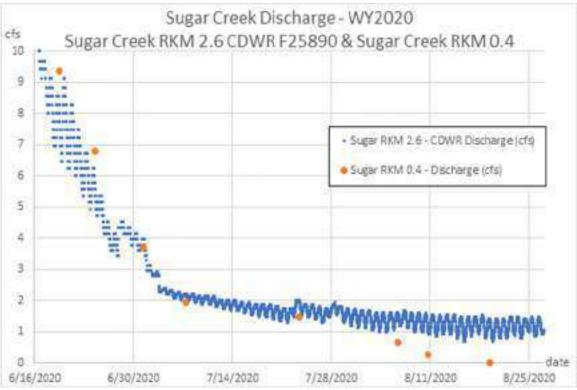
Figure 27. Continuous discharge (cfs) at CDWR RKM 2.6 station and periodic discharge are RKM 0.4.
