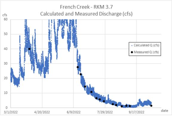
Figure 1 – Calculated and measured discharge (cfs) – French Creek RKM 3.7
