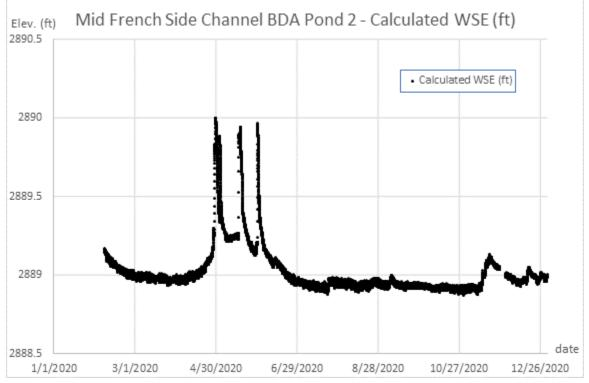
Figure xx – Calculated Water Surface Elevation (WSE) – Side Channel BDA Pond 2
