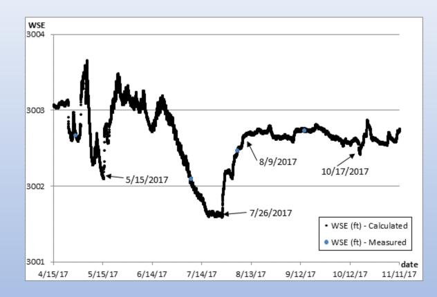
Water Surface Elevation in Sugar BDA 1 Pond – WY 17
