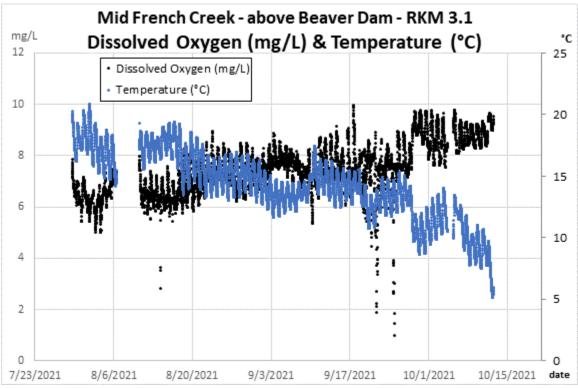
Figure 5 - Dissolved oxygen (mg/L) and temperature (°C)
