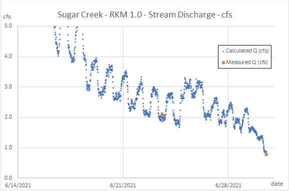
Figure 1 – Calculated and measured discharge (cfs) – Sugar Creek RKM 1.0
