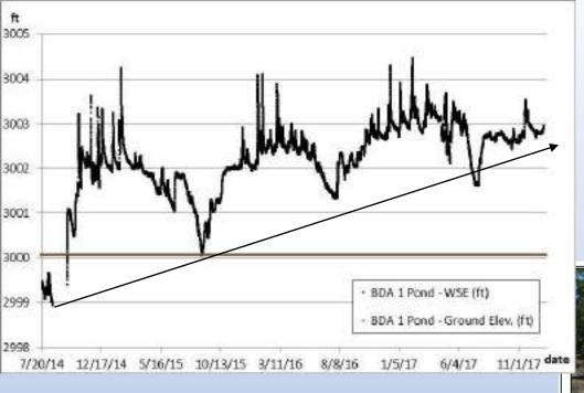
Water surface elevation during the base flow period of summer has increased every year since the installation of the BDAs in Lower Sugar
