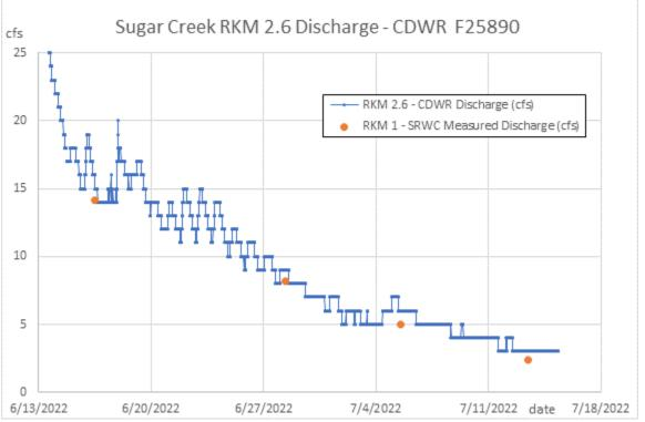
Figure 3 – Continuous discharge at Sugar RKM 2.6 and periodic discharge at RKM 1.0 – WY2022
