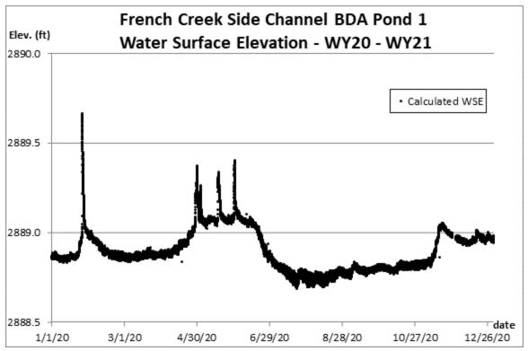
Figure xx – Calculated Water Surface Elevation (WSE) – Side Channel BDA Pond 1
