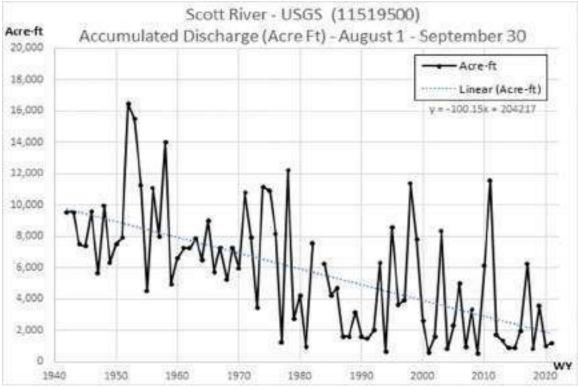
Figure 5. Accumulated discharge (af) – August 1st through September 30th.
