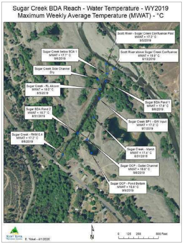
Figure 11. Maximum MWAT (°C) and date of occurrence during base flow - WY2019.
