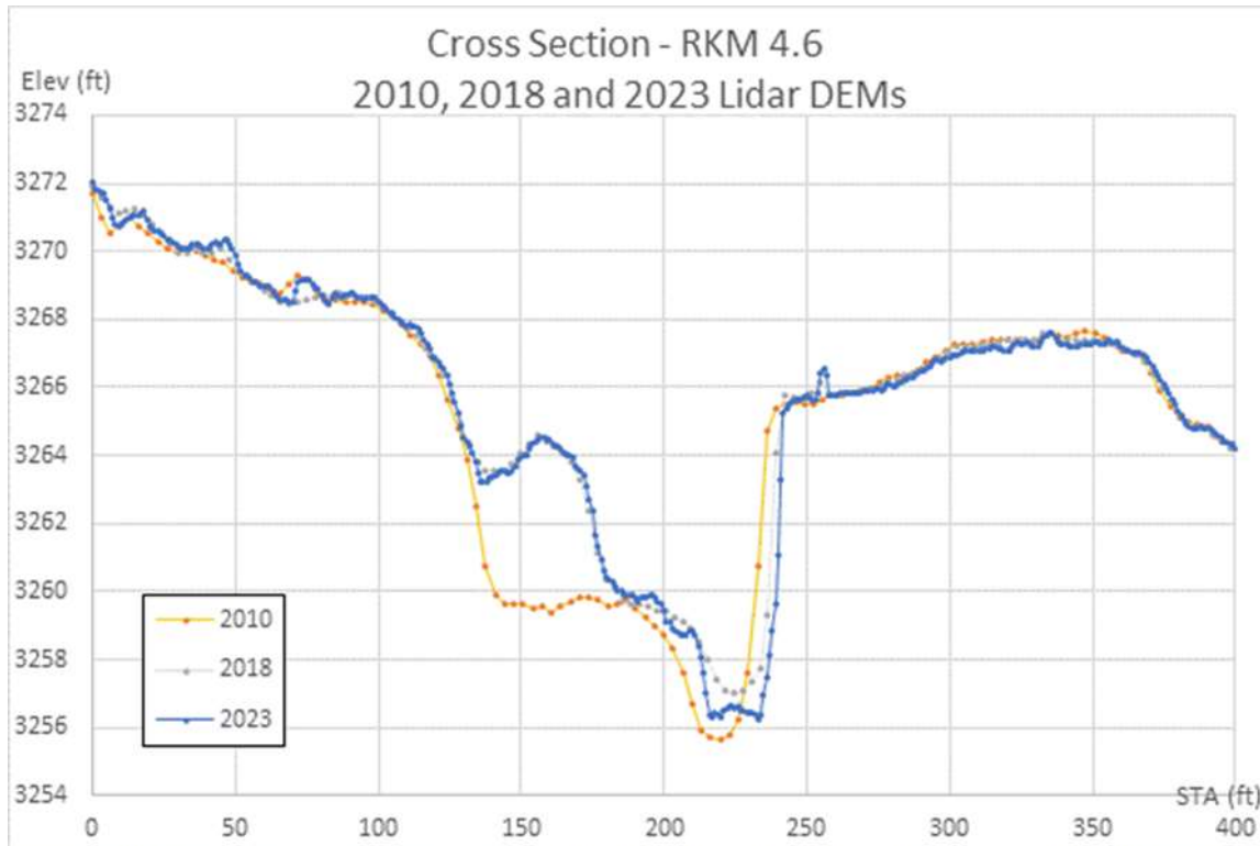
Figure 8 - 2010, 2018 and 2023 LiDAR Cross Section - East Fork Scott River RKM 4.6
