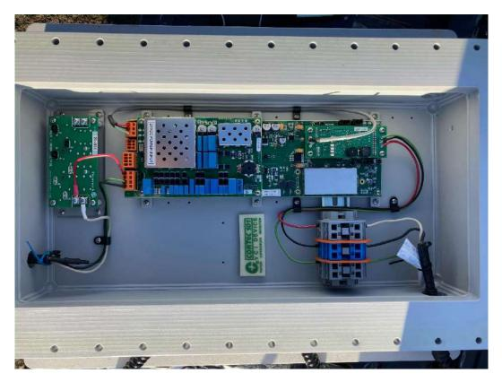
Picture 3. Fishway enclosure housing IS1001 reader and capacitance board.
