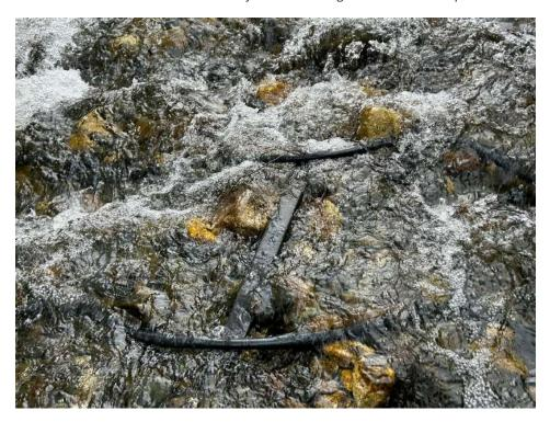
Picture 6. Flexible antenna lying flat on streambed at French Creek downstream array.
